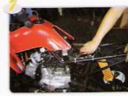
Cut off the elec. Wiring tie-down
