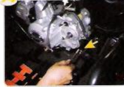
Unplug the starter wiring
